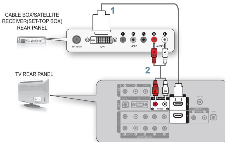
1. Connect an HDMI Cable(Not supplied) between the **HDMI IN 2** jack on the TV and the HDMI jack on the Cable Box/Satellite receiver (Set-Top Box).
